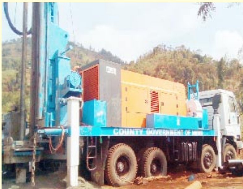
A rig machine purchased by county government to sink boreholes.
